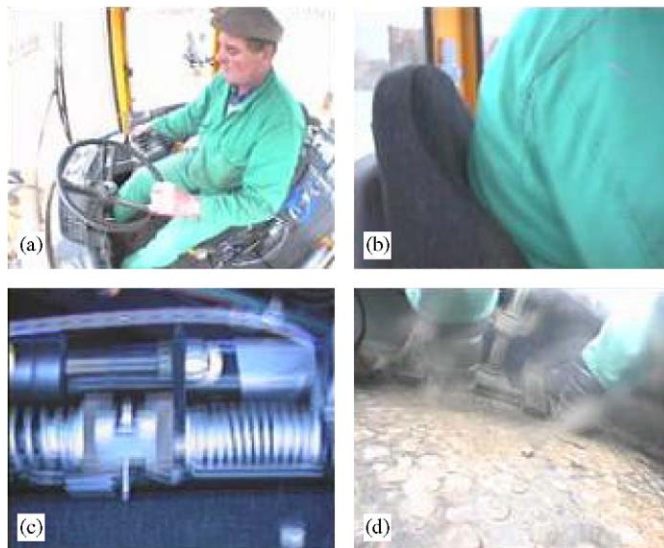
Fig. 3. The four views recorded in the cab: (a) hand location; (b) contact area back/backrest; (c) fore-and-aft suspension; (d) foot position.
