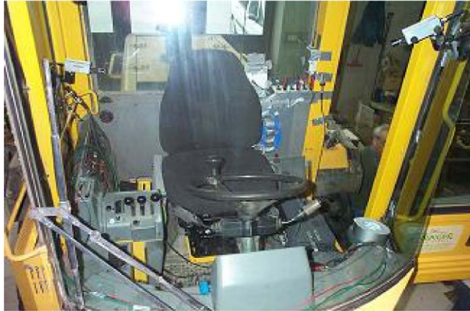
Fig. 2. Instrumentation of the cab with accelerometers and cameras.
