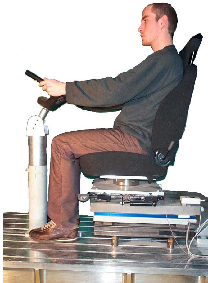
Fig. 8. Seat mounted on a shaker to measure the apparent mass of a seated subject.
